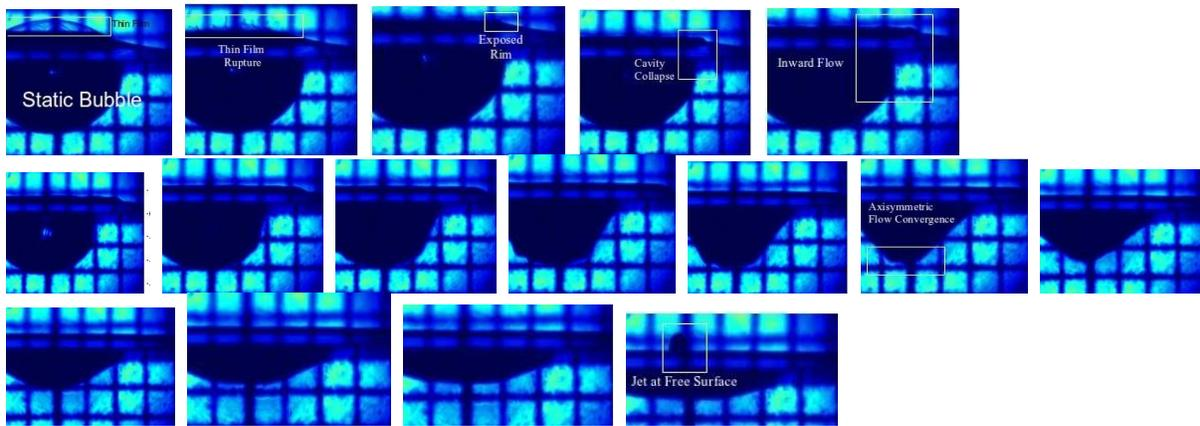
Fig 3: Different stages of bubble burst (from left to right) for bubble radius  $R = 2.1852$  mm @3000 fps, grid size is 1 mm
