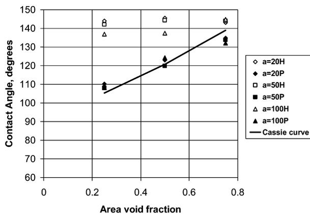
**Figure 3.** Contact angle versus area void fraction for varying characteristic lengths ( $D = 30 \mu\text{m}$ ).
