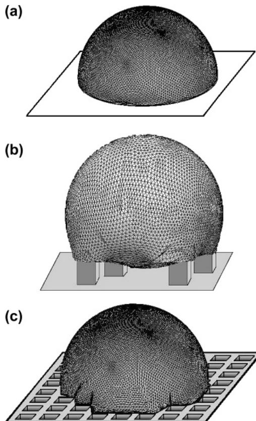
**Figure 1.** (a) Shape of a sessile drop on a smooth surface generated using Evolver.<sup>26</sup> (b) Shape of a sessile drop on a surface with square poles generated using Evolver.<sup>26</sup> (c) Schematic of a sessile drop on a surface with square holes.
