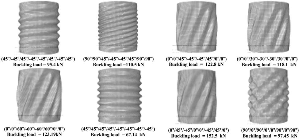
Fig. 2 Mode shapes and buckling loads for different lay up sequences
