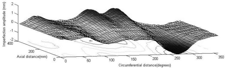
Fig. 4 Variation of initial imperfection of the outer surface of the cylindrical shell specimen 2
