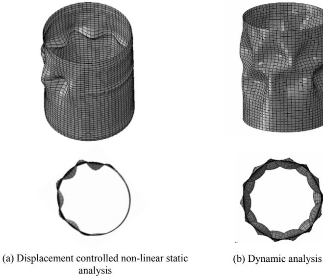
Fig.10. Buckling Modes of the Specimen 2 under displacement control
