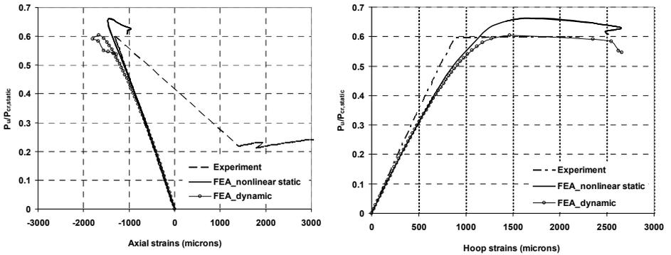
Fig. 13 Comparison of the axial and hoop strains with axial load (Specimen 2)
