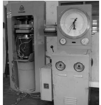
Fig.5. Final set up for the load controlled static buckling test
