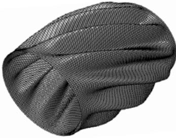
(a) Linear buckling analysis,  $P_{cr} = 165.77$  kN
