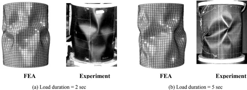
Fig.14 Buckling modes obtained under dynamic loading for different time durations
