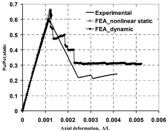
Fig. 12 Comparison of axial load vs. axial deformation (non-dimensional) for Specimen 2
