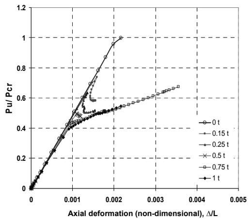
(b) Variation of axial load with axial deformation (non-dimensional) for various imperfection amplitudes ( $\delta_0$ )
