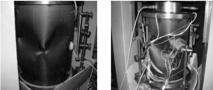
Fig.6 Buckling modes obtained in the load controlled test
