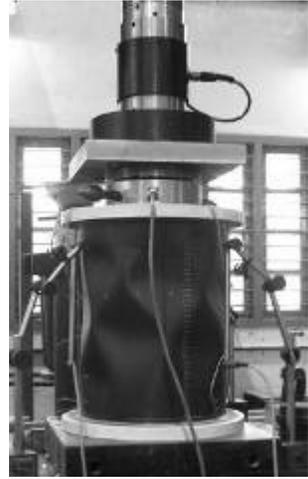
Fig. 7 Buckling mode under displacement controlled static buckling test
