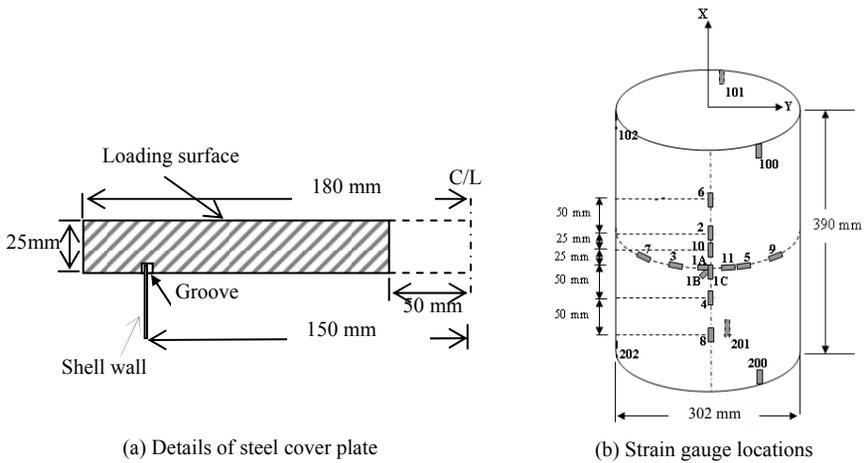
Fig.3. (a) The details of the covering plates attached to the top and bottom of the shell.
