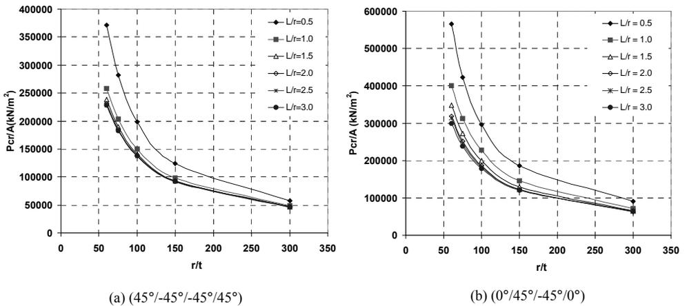
Fig.1 Variation of  $P_{cr}/A$  for various  $L/r$  and  $r/t$  ratios for two different lay-up sequences
