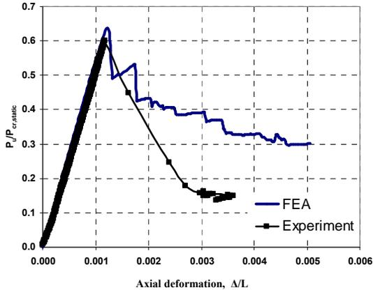
Fig. 15. Comparison of Axial load Vs Axial displacement for Specimen 4
