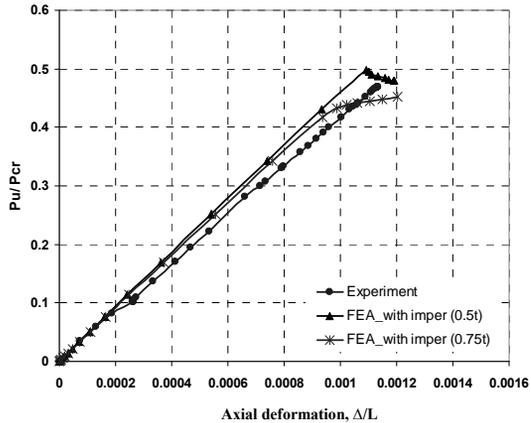
Fig. 11. Comparison of the Load Vs Axial deformation (non-dimensional) plots obtained from FEA for the specimen 1 for different imperfection amplitudes with the experiment.
